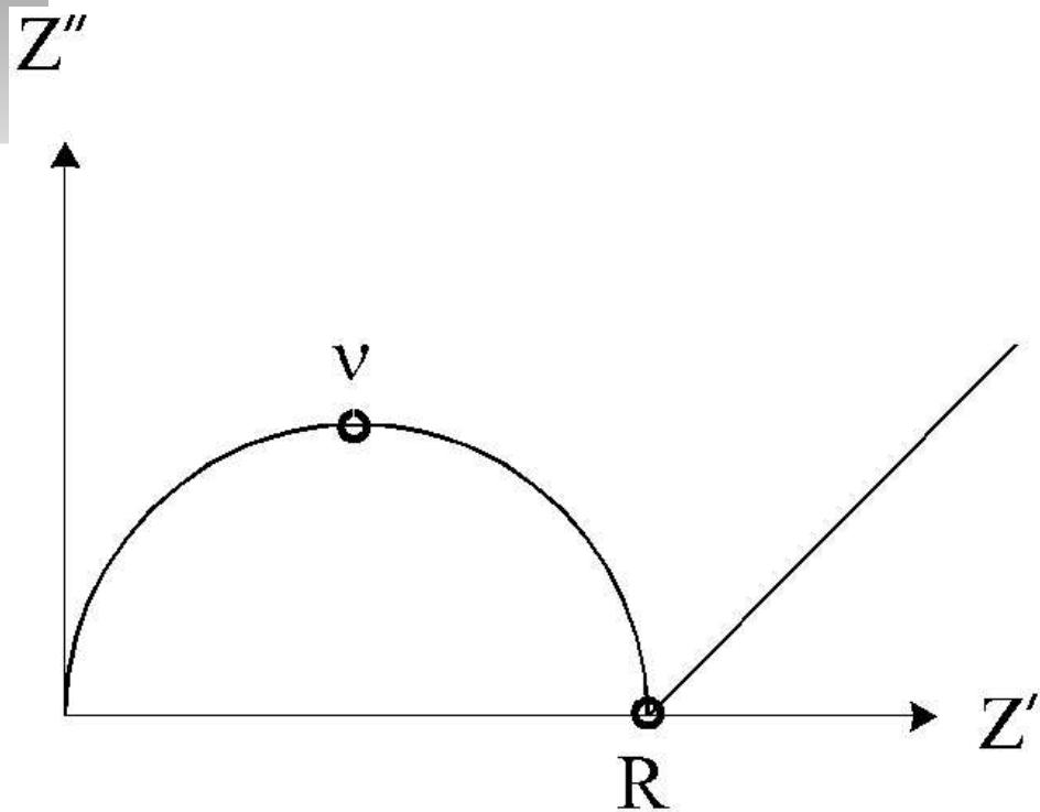
R: Resistance of the ohmic resistor of one parallel circuit  $R = Z'$
