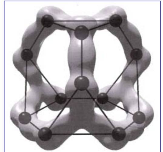
Diffusion path of \text{Ag}^+ ions in a silver ionic conductor
