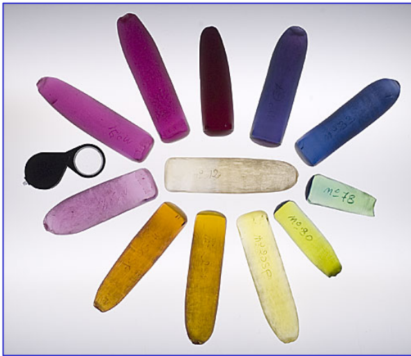
Synthetic corundum crystals obtained by the Verneuil process
