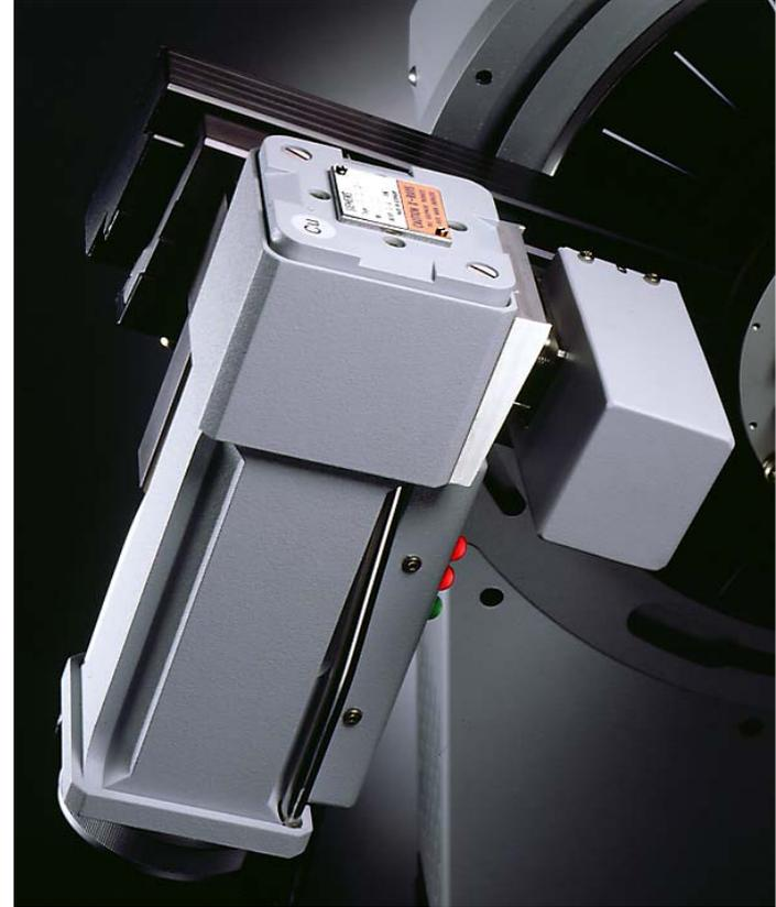
X-ray tube with shielding
