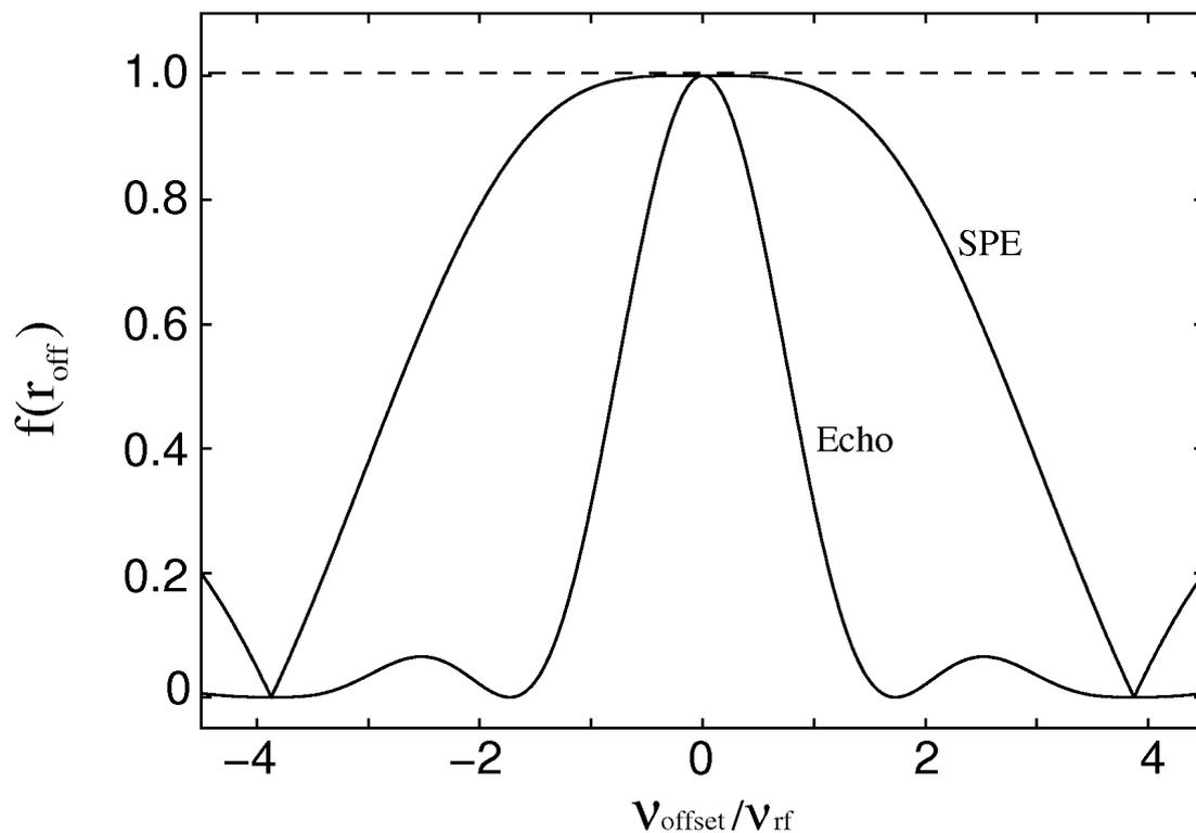
**Figure 5:** Signal yield as a function of the offset factor  $\nu_{\text{off}}/\nu_{\text{rf}}$  of a single pulse excitation experiment (SPE with a pulse with  $90^\circ$  flip angle) and a spin-echo experiment (Echo);  $\nu_{\text{off}}$  is the difference between transmitter frequency and Larmor frequency,  $\nu_{\text{rf}}$  is the pulse nutation frequency  $\nu_{\text{rf}}$  (see text).
