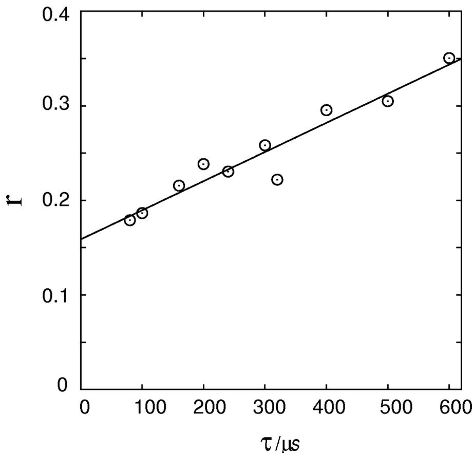
**Figure 4:** Experimental peak area ratio as a function of the spin-echo delay  $\tau$  (see Figure 3) for a mixture of adamantane and ammonium dihydrogenphosphate (mixture 5, see Table 1) determined by  $^1\text{H}$  MAS NMR; the solid line was obtained by linear regression; experimental conditions (case III, see text): sample spinning speed  $\sim 25$  kHz, magnetic field of 4.7 T.
