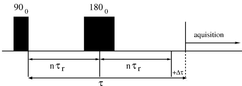
**Figure 3:** Modified rotor-synchronized spin-echo pulse sequence used for quantitative measurements;  $\tau_r$  designates a rotor period,  $\Delta\tau$  is a small delay which has to be determined once so that (small) first order phase corrections become unnecessary; these are caused by finite pulse effects and hidden delays in the receiver of the NMR spectrometer.
