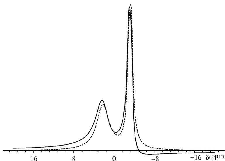
**Figure 1:** Simulated NMR spectra of a line shape function perfectly in phase (dotted line) and a lineshape being out of phase (signal phase  $\phi = 10^\circ$ ) but with otherwise identical lineshape parameters.
