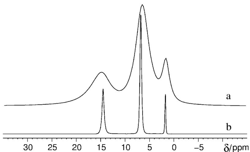
**Figure 2:**  $^1\text{H}$  MAS NMR spectra of a mixture of adamantane and ammonium dihydrogenphosphate obtained at (bottom to top) 65 kHz and 25 kHz sample spinning speed, respectively; spectrum (b) was recorded at 600 MHz and spectrum (a) was recorded at 200 MHz resonance frequency.
