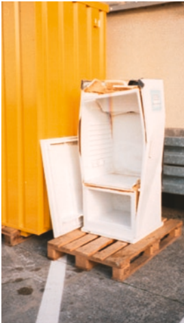
Picture 12: Consequences of using a fridge that was not explosion-proof
