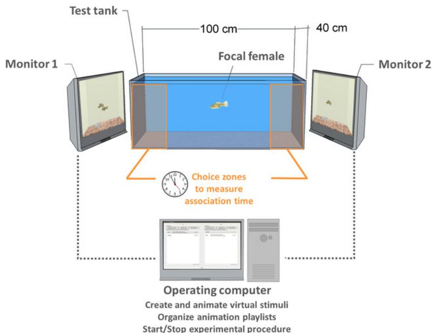
**Figure 6: Experimental setup for the MCC experiment with computer animation.** The operating computer connects to two presentation monitors (Monitor 1 and 2) which replay animations to live focal females inside the test tank. For illustration, both LCD monitors are angled to show an animated scene. [Please click here to view a larger version of this figure.](#)
