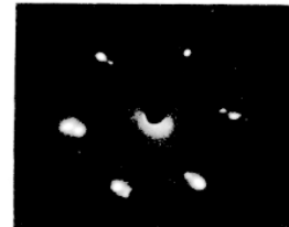
assignment of LEED pattern to defect density of platinum surface
