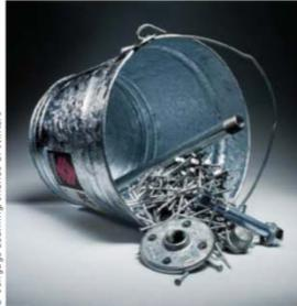
Galvanized objects are made of steel that is coated with zinc to protect against corrosion.
