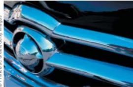
Steel is plated with chromium for appearance as well as protection against corrosion.
