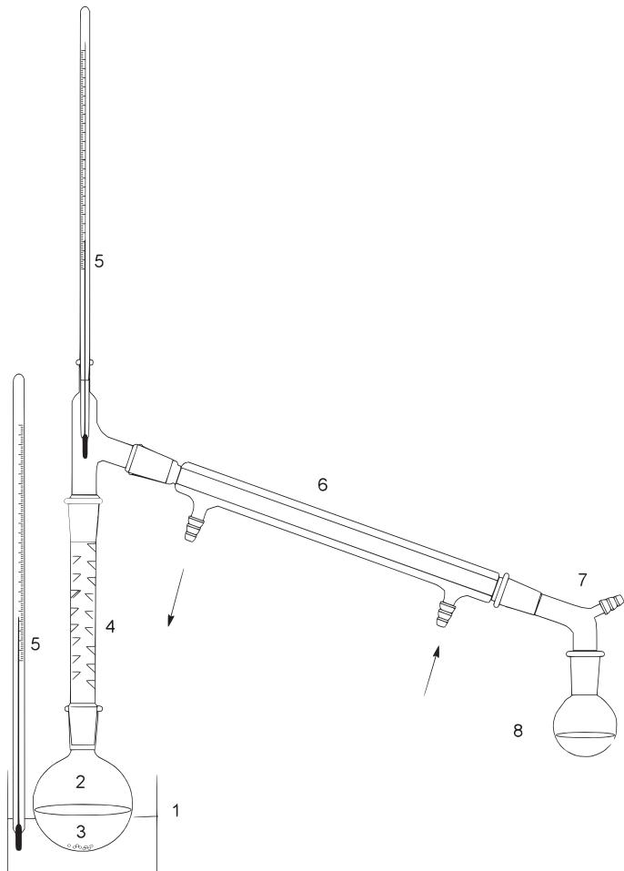
**Abb. 3.5:** Die aufzubauende Destillationsapparatur: 1: heating bath, 2: Distillation flask, 3: boiling chips, 4: Vigreux column, 5: Thermometer, 6: Liebig cooler, 7: Vakuum feed, 8: receiver
