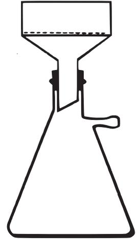
**Abb. 3.4:** sucking flask with suction strainer
