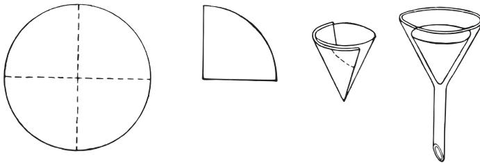
**Abb. 3.2:** Folding of paper filters
