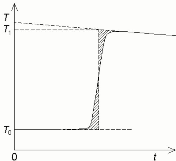
**Abb. 7.2:** Temperature profile when determining the heat of solution
