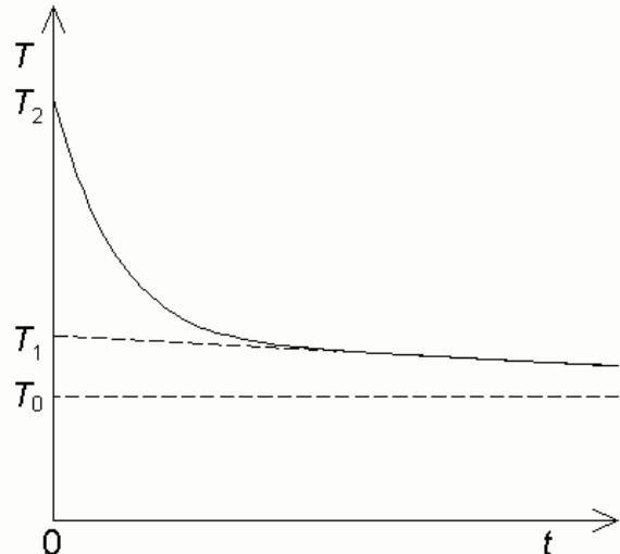
**Abb. 7.1:** Temperature change when determining the heat capacity
