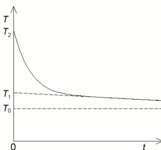
**Abb. 7.1:** Temperature change when determining the heat capacity
