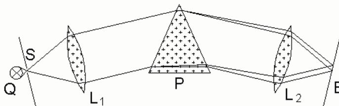
**Abb. 4.2:** Beam path in the spectroscope
