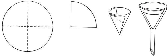
**Abb. 3.2:** Folding of paper filters
