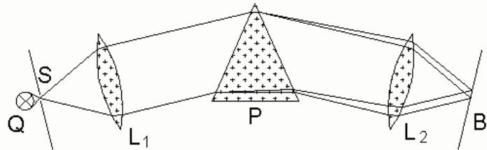
**Abb. 4.2:** Beam path in the spectrometer
